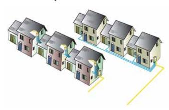
A significant majority of new condominiums and town homes are constructed using a horizontal layout that very closely resembles the arrangement of single family homes. Because of the similarity of single family homes the FTTP connector scheme is often identically equivalent. Usually the network interface will be a Fiber Distribution Terminal located on the exterior surface of the structure.
